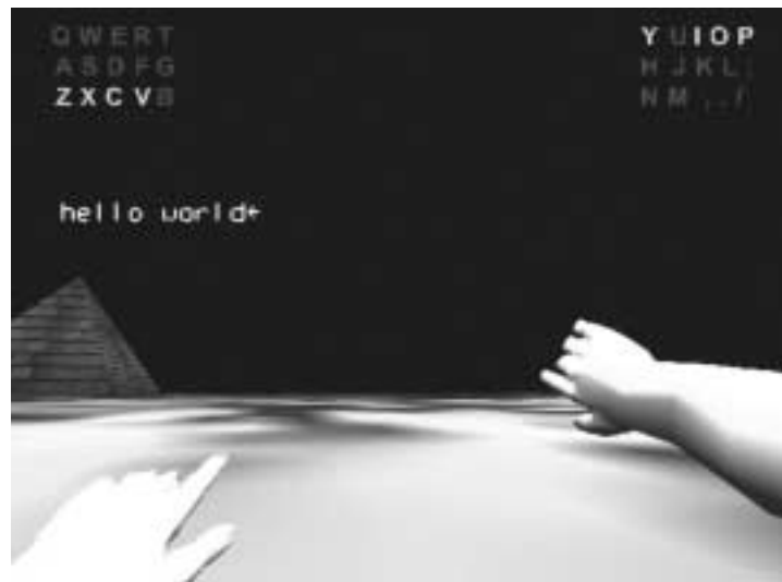
Figure 9.2 User's view of the Pinch Keyboard. (Bowman, Wingrave et al. 2001, © 2001 by Springer-Verlag; reprinted with permission)
