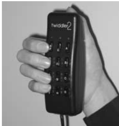
Figure 9.1 A 12-key chord keyboard. (Photograph courtesy of Doug Bowman)
