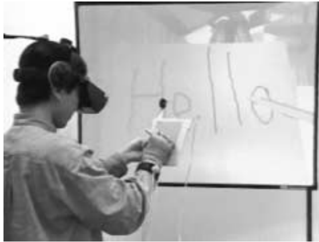
Figure 9.6 The Virtual Notepad system allowing handwriting in an immersive VE. (Poupyrev, Tomokazu et al. 1998, © 1998 IEEE)
