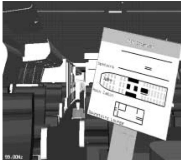
Figure 10.10 Embedding an interactive 2D interface into a 3D VE. (Angus and Sowizral 1996, © 1996 IEEE)
