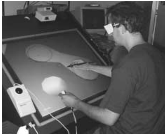
Figure 10.13 Sketching 3D objects directly on the display surface in Ergodesk. (Forsberg et al. 1997, © 1997 IEEE)
