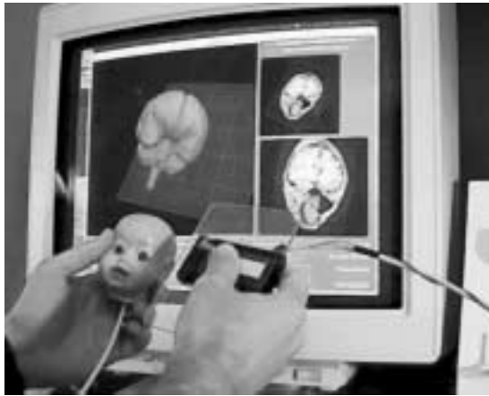
Figure 10.2 Two-handed interface with passive haptic feedback provided by the doll head and cutting plane tool held by the user. (Hinckley et al. 1994, © 1994 IEEE)
