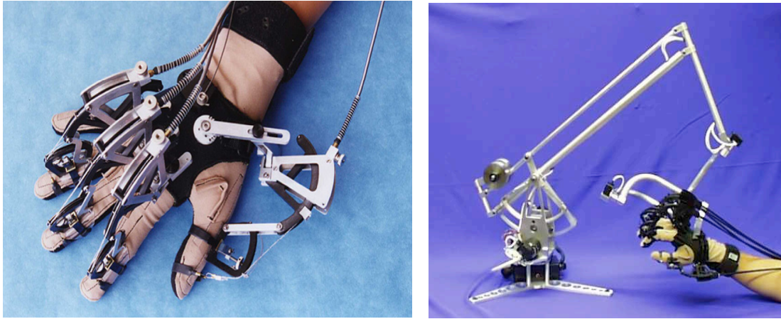
Figure 8: Exoskeleton (left) and combination exoskeleton and mechanical linkage (right) haptic devices from Virtual Technologies, Inc.
