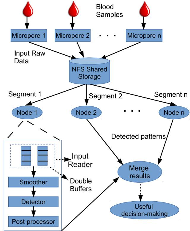
Figure 1. Distributed Detection Framework: Data can be collected from multiple bio-nano sensors on a shared storage of a high-speed server. Clusters nodes retrieve their own data segment from the shared storage and process it in parallel. Each data segment is processed by an individual node in four steps, including pre-processor, smoother, detector, and post-processor that delivers results for useful decision-making.
