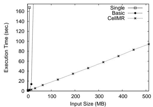
Figure 7. K-Means execution time with increasing input size.
