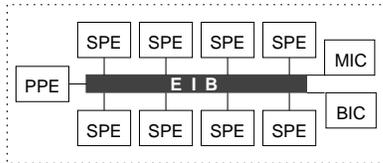
Figure 1. Cell architecture.
