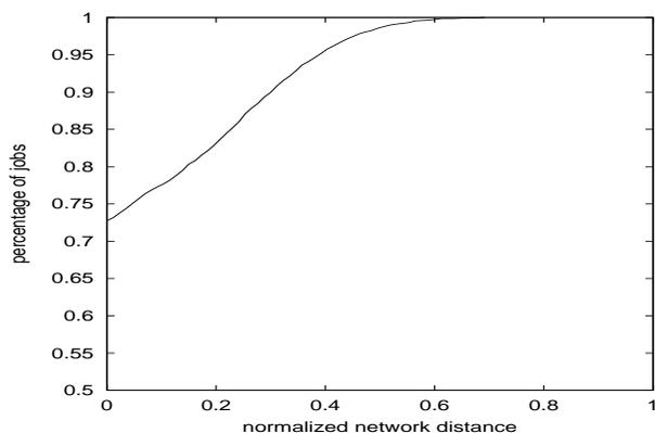
**Figure 6: Cumulative distribution of locality for scheduled jobs when flocking is enabled. The x-axis stands for the ratio between the network distance from the job submission pool to the actual execution pool and the diameter of the underlying IP network. Locality zero means that the jobs are scheduled inside local Condor pools.**
