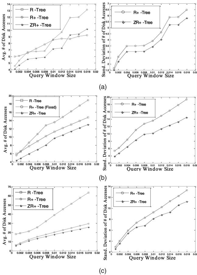
Fig. 11. Window query performance of R-tree, R+-tree, and ZR+-tree. (a) Window query on major roads of Germany. (b) Window query on roads of Long Beach County. (c) Window query on synthetic data.
