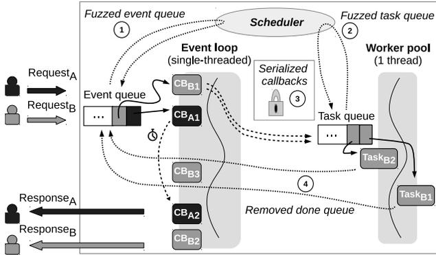
**Figure 5.** Highlights of *Node.fz*, our fuzzed EDA scheme, targeting AMPED architectures like Node.js. This figure illustrates the same case as Figure 1, with many callback orderings changed by the scheduler. Dotted lines indicate architectural changes compared to Figure 1.
