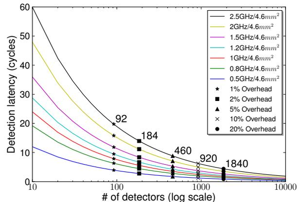
**Figure 1.** Soft error detection latencies varying the number of sensors under the configurations of ARM cortex-A9 out-of-order processors where the core part takes a quarter of total die size.
