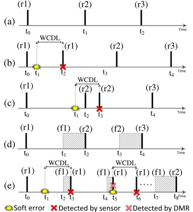
**Figure 2.** Problem of idempotent processing in the presence of the sensor-based soft error detection scheme and its worst-case detection latency (WCDL), and our tail-DMR solution.
