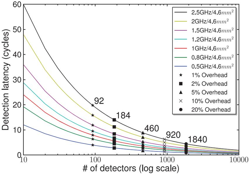
Fig. 1. Soft error detection latencies varying the number of sensors under the configurations of ARM cortex-A9 out-of-order processors where the core part takes a quarter of total die size.
