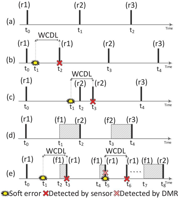
Fig. 2. Problem of idempotent processing in the presence of the sensor-based soft error detection scheme and its worst-case detection latency (WCDL), and our tail-DMR solution.
