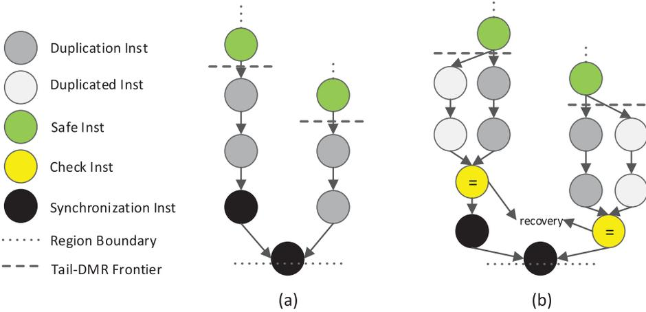
Fig. 4. Tail DMR-frontier and code duplication example: (a) an example control data flow graph with tail-DMR frontiers and (b) code duplication performed by Clover.
