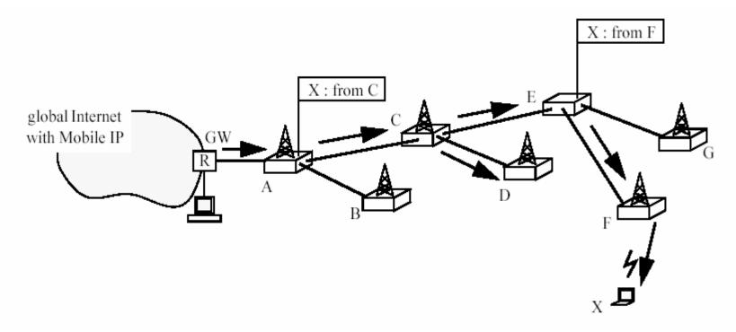
When IP packets arrive at the GW, addressed to a MH for which no up-to-date routing information is available, the gateway queues the arrived IP packets and generates a *paging packet*
