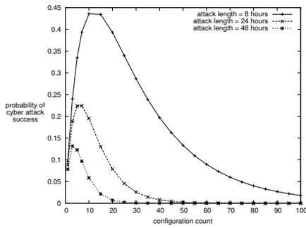
Fig. 3. Probability of cyber attack success versus configuration count and cyber attack length (closed-form model).
