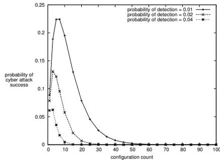
Fig. 10. Probability of cyber attack success versus configuration count and probability of implant detection (stochastic model).
