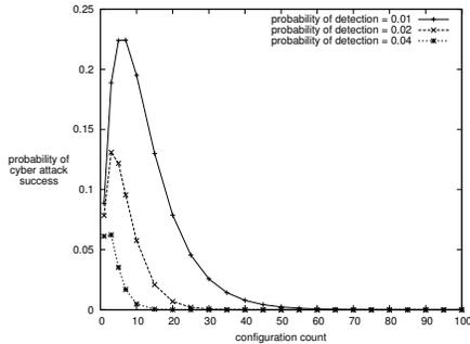
Fig. 6. Probability of cyber attack success versus configuration count and probability of implant detection (closed-form model).
