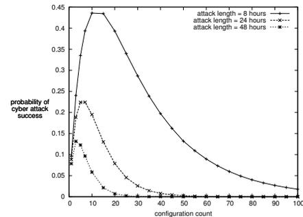
Fig. 7. Probability of cyber attack success versus configuration count and cyber attack length (stochastic model).
