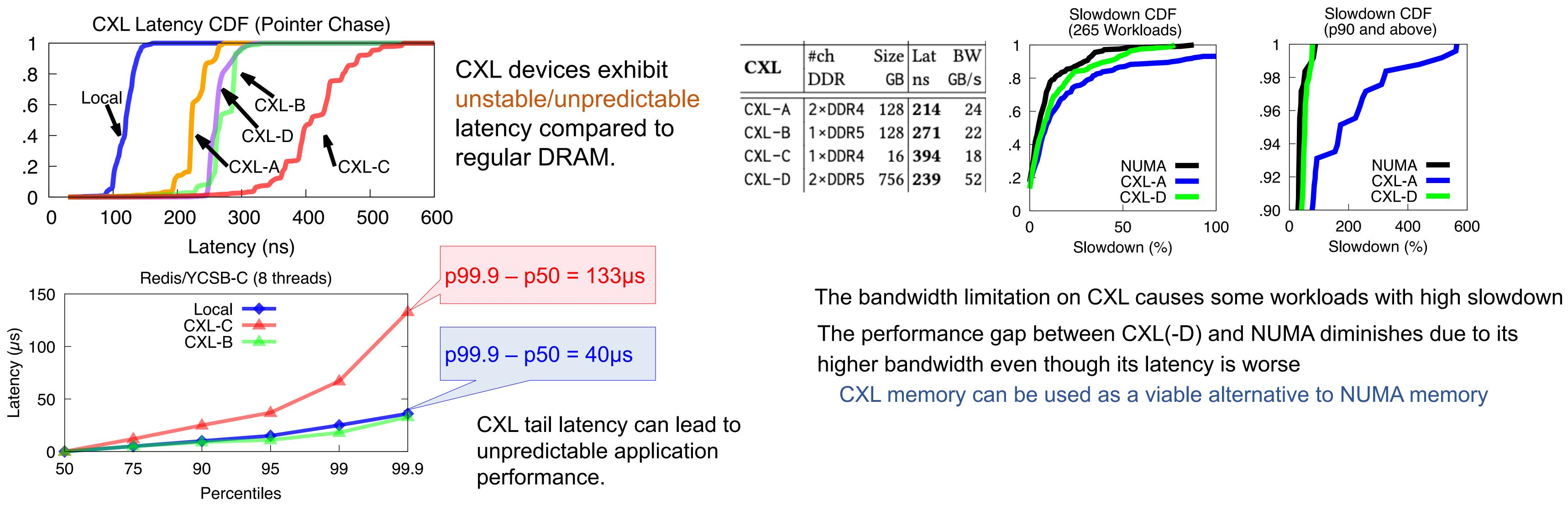
The performance gap between CXL(-D) and NUMA diminishes due to its CXL memory can be used as a viable alternative to NUMA memory
