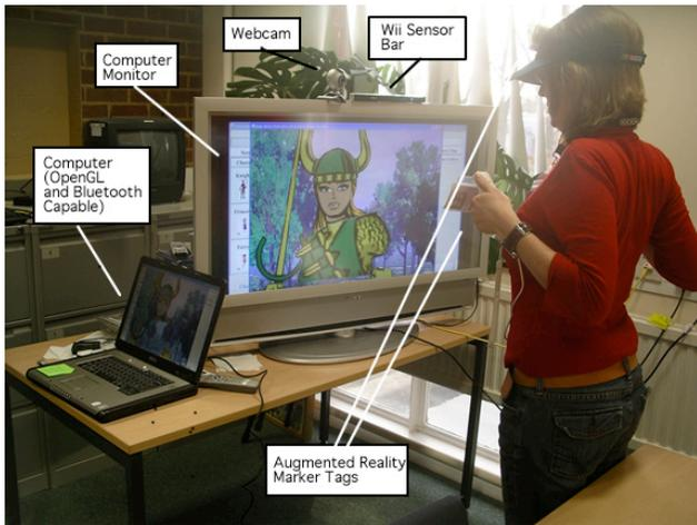
**Figure 1. The STAGE prototype**
