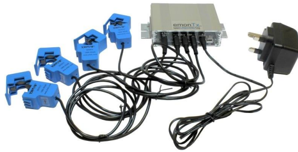
Figure 10 EmonTx; Power Monitor
