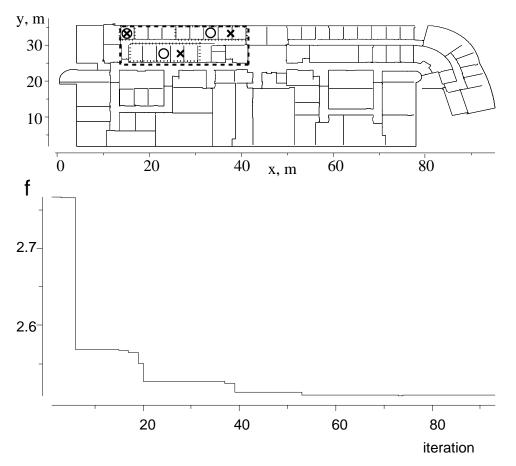
Power coverage optimization results for three transmitters. The starting (optimal) locations are marked with circles (crosses).
