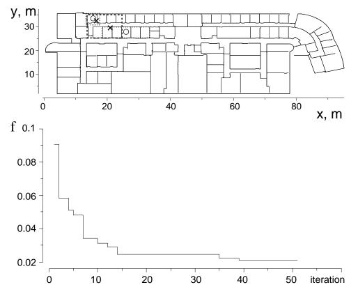
BER optimization results for two transmitters. The starting (optimal) locations are marked with circles (crosses).
