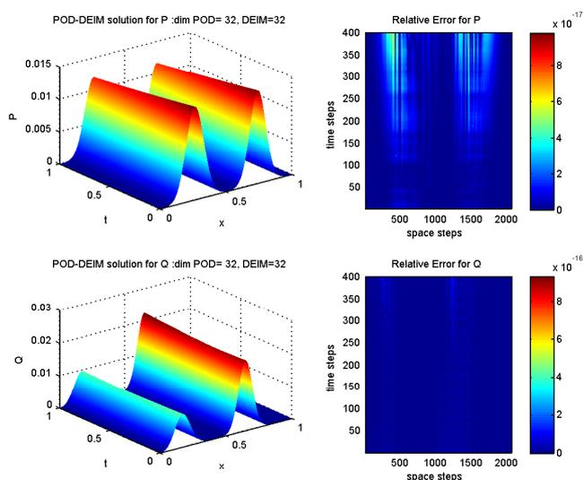
Figure 4: Solution plots ( $P, Q$ ) of the model from POD-DEIM reduced system ( $\dim\text{POD}=\dim\text{DEIM}=32$ ), with the corresponding average relative errors at the inner grid points ( $n = 2048$ ).
