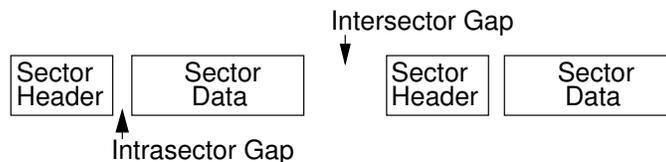
**Figure 8.4** An illustration of sector gaps within a track. Each sector begins with a sector header containing the sector address and an error detection code for the contents of that sector. The sector header is followed by a small intra-sector gap, followed in turn by the sector data. Each sector is separated from the next sector by a larger inter-sector gap.
