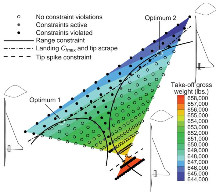
Figure 2. A 2D slice through a multidimensional parameter space using the points Optimum 1 and Optimum 2 and another suboptimal feasible point.
