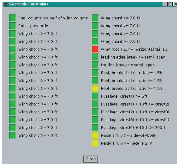
Figure 4. Geometric constraints for one design point. A red box indicates a violated constraint, a yellow box indicates an active constraint, and a green box indicates a satisfied constraint.
