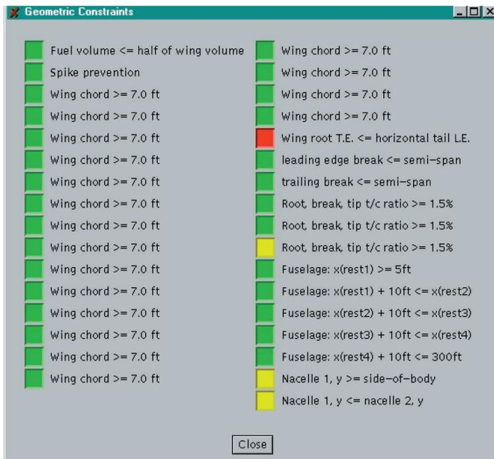
Figure 4. Geometric constraints for one design point. A red box indicates a violated constraint, a yellow box indicates an active constraint, and a green box indicates a satisfied constraint.
