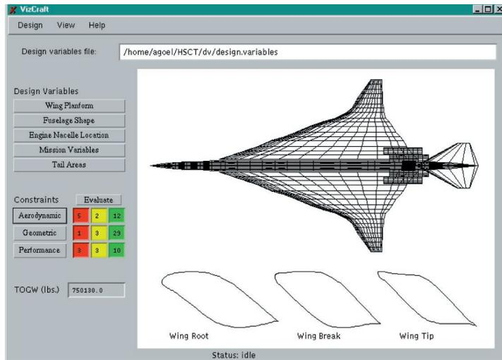
**Figure 1.** A VizCraft design view window showing aircraft geometry and cross sections of the airfoil at the root, leading edge break, and wing tip.
