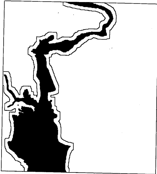
Figure 8. An example of the WITHIN function: expansion of the floodplain by 8 units.
