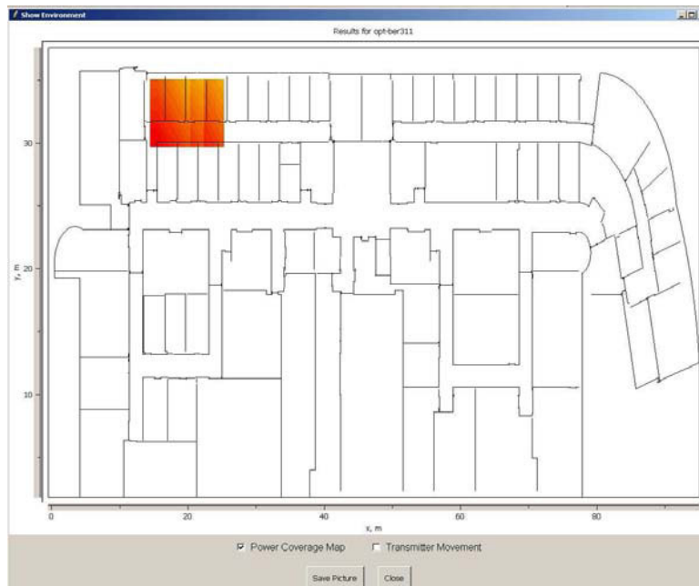
Figure 8. Visualization of power coverage on the environment map. Intensity of the color is proportional to the power level.
