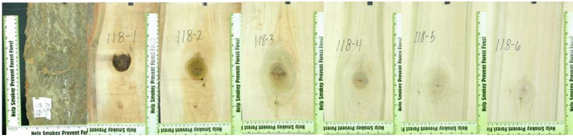
Figure 1.—Photo series showing processed defect sample
