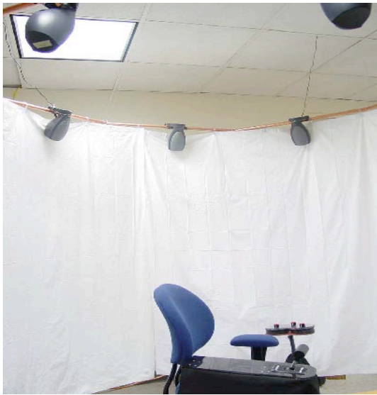
Fig 7. LOUD is a selection interface to a library of music. It is intended to aid in the identification of genre, performer, beat, instrument, and other aspects by rotating in the chair to face one of four different channels. Students hand-built a coarse rotary shaft encoder to sense the direction of the chair. The most complex system architecture among the four projects, four stereo playback channels selected from an aspect database of musical selections.
