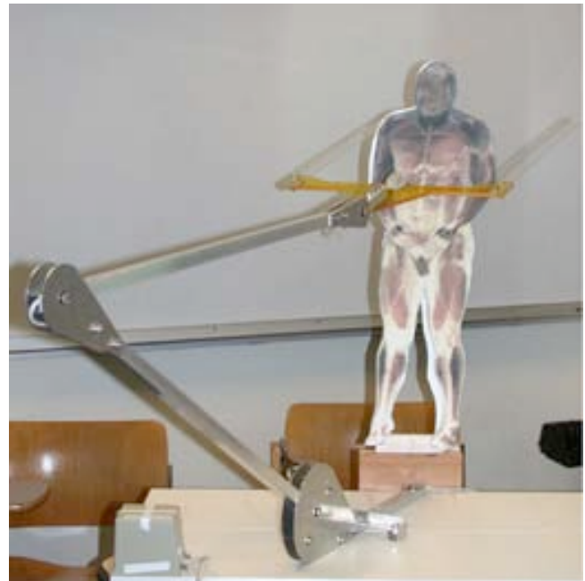
Fig 7. Eeeww! used a repositionable wand to show where the virtual slice is made. It is intended for middle school human biology classes. The project name was suggested by users brought in to evaluate the project. It also used the Flock Of Birds sensor.
