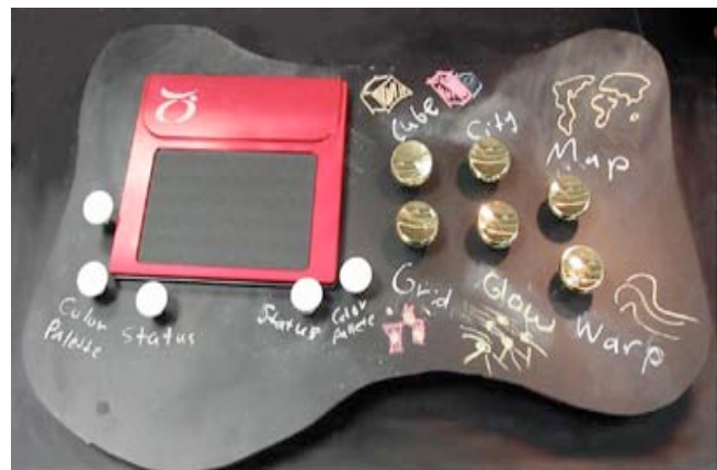
Fig 4. Shazam. A digital light show system. The controller is a chalkboard so that buttons can be annotated with notes or drawings of effects associated with them. The TacTex pad works and a rhythm wand (not shown) are used to set beat and modulate visual effects. Selected for the AIGA LOOP Award.
