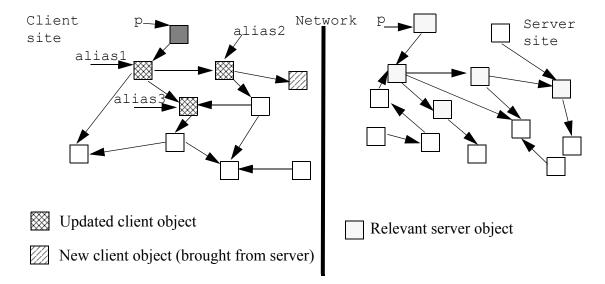
**Figure 8-1:** (b): A general remote call mechanism: param p is returned to the client and restored in place.
