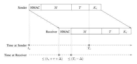
Fig. 2. Timing of a packet in transmission using TIK
