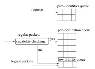
Figure 2: Queue management at a capability router. There are three types of traffic: requests that are rate-limited; regular packets with associated capabilities that receive preferential forwarding; and legacy traffic that competes for any remaining bandwidth.
