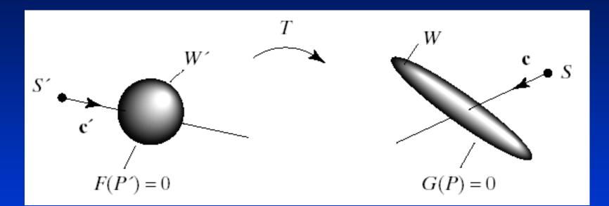
• Where does S+ct hit the transformed sphere G?
